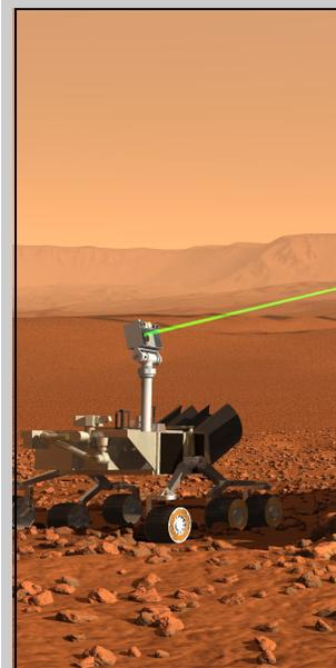
The Curiosity ChemCam uses a laser for much of its information gathering. Illustration source: Los Alamos National Laboratory
