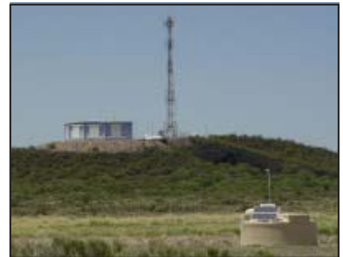
At Auger South: On the hill is a fluorescent power building and a communications tower. In the foreground is a typical surface detector tank.
